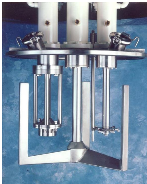
Fig.12. Triple Shaft Mixers: one shaft with rotor-stator impeller (left), one with anchor vanes (center) and one shaft with High-shear impeller. Each shaft is operated and moved independently of the others
