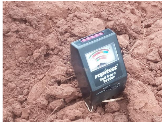
Fig.1. Rapitest 4-in-1 soil tester
