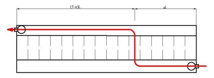
**Fig.5.** Representation of the flow along the vertical orthogonal plane at a distance xL from the entrance to the upper honeycomb
