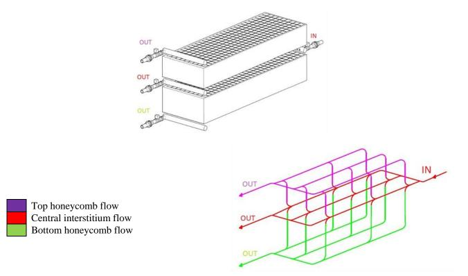
Fig.7. 3D graphic representation of the interaction of flows inside the GSMF separator
