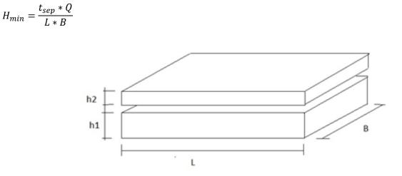
Fig.3. Main dimensions of the two honeycomb packs
