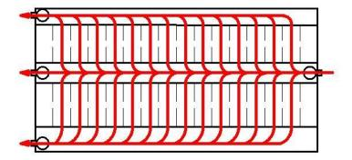
Fig.6. Representation of the flows on the vertical orthogonal plane for each transverse row of shafts
