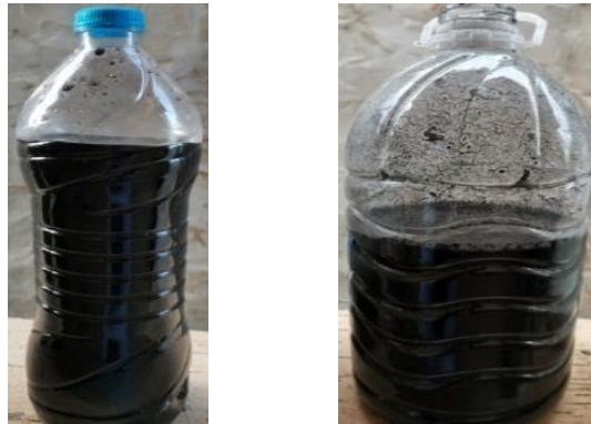
Fig.3. Sample of treated wastewater with using Charcoal
