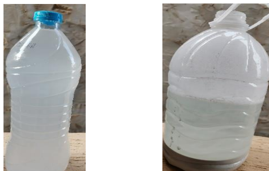
Fig.4. Sample of treated wastewater with using Lime
