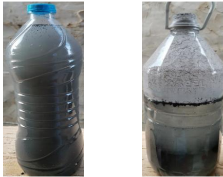
Fig.5. Sample of treated wastewater with using Lime and Charcoal
