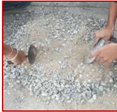
Figure 3. Mixing of Concrete and Waste Foam Plastic.
