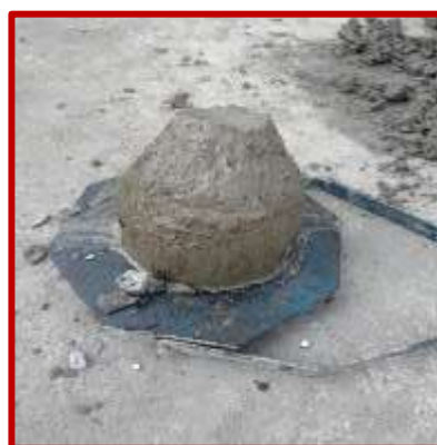
Figure 2. Failure of Slump Cone.
