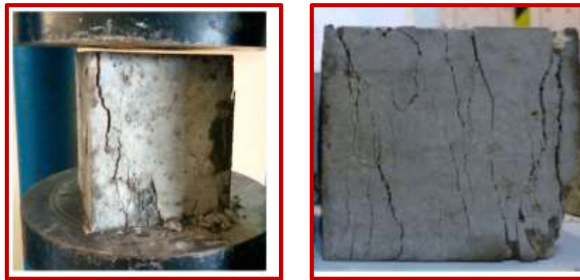
Figure 6. Cube Failure on Load.
