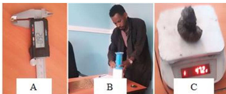
Figure 1. Determination of various physical properties of barley grains
