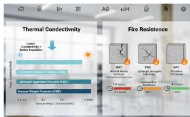
Figure 2. Comparison of thermal conductivity and fire resistance of concrete types [12-14].
