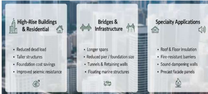
Figure 4. Applications of lightweight concrete in buildings and infrastructure [18-20].
