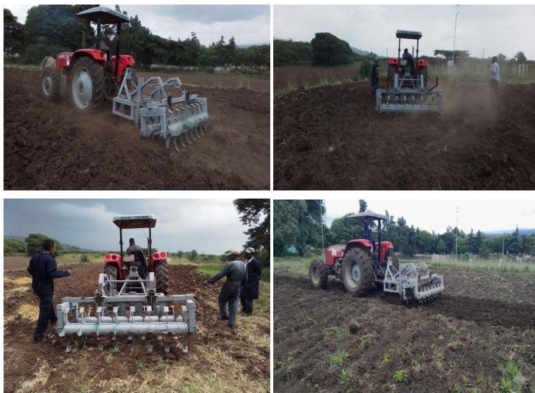
Figure 1. Operation during performance evaluation of combined tillage implement
