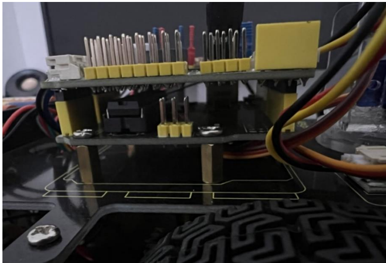
Figure 2. The Arduino UNO-type board on the base under the shield in the construction [11]
